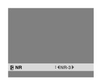
\* If neither the ◀ or ► button is pressed within 5 seconds, the current selection is set and the previous screen reappears. 4. Press the "PROCEED" button. The noise reduction mode is set to "NR-3".
